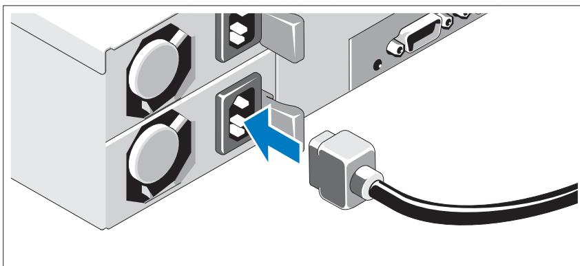
Connect the system's power cable(s) to the system and, if a monitor is used, connect the monitor's power cable to the monitor. Plug the other end of the power cables into a grounded electrical outlet or a separate power source such as an uninterrupted power supply (UPS) or a power distribution unit (PDU).
